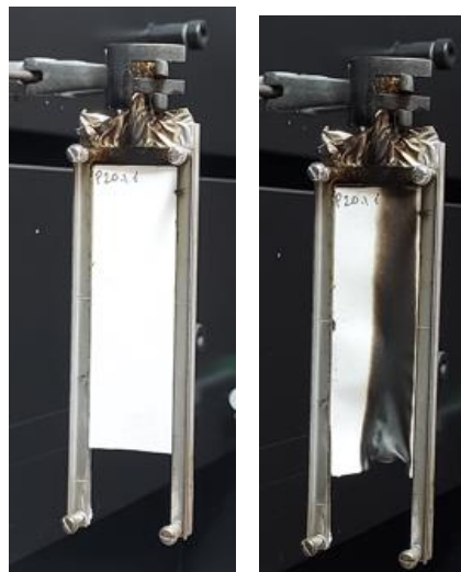
Figure 3. Paper treated with phytic acid before (left) and after (right) UL94 test.
