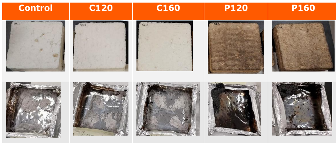
Figure 4. Visual appearance of the foams before (top row) and after (bottom row) the cone calorimeter test.
