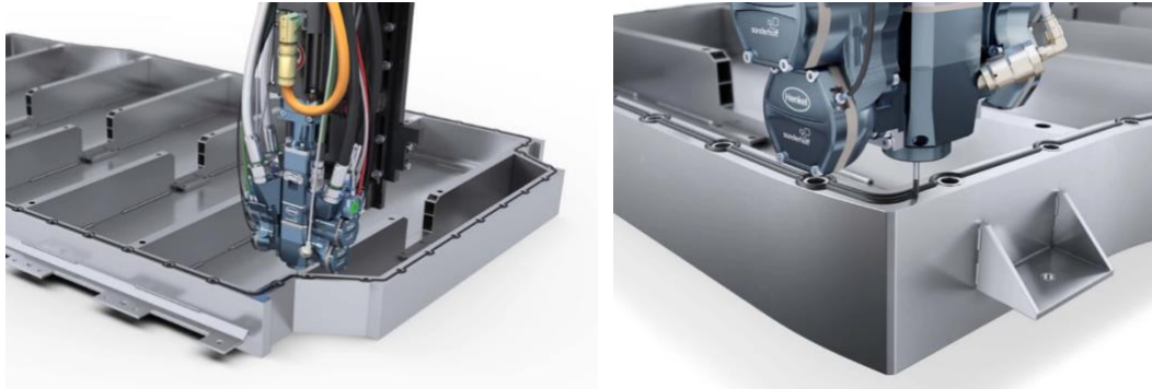
Figure 10: Automated application of rubber sealant on battery pack housing (and close-up) [102]
