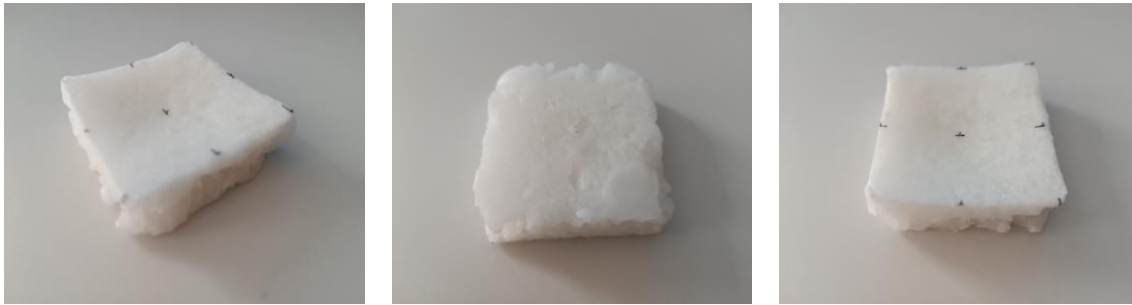
Figure 23: Frothed BreadCell foam saturated with liquid Paraffin, in solid state (transition temperature 60°C): 3g of Paraffin per gramm foam
