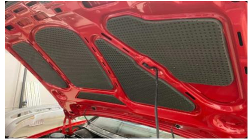
Figure 5: Tailor-made PUR-insulation panels for bonnet [82]
