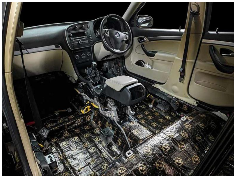
Figure 7: Aftermarket noise insulation PE foam mats from "Standartplast" applied to interior floor [95]
