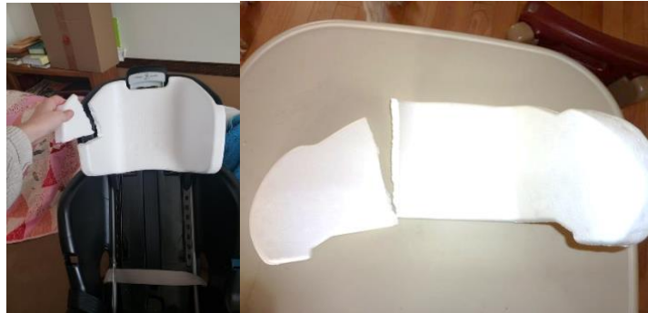
Figure 17: Foam impact liner ripped off (fabric cover removed); Source: [159,160]
