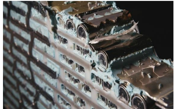
Figure 6: Example of silicone-foam (cyan) encapsulation of Tesla battery pack after dismatling for examination [90]
