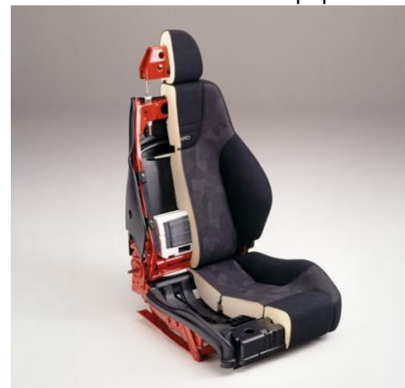
Figure 2: Foam cushions give the seat its form and function [1]
