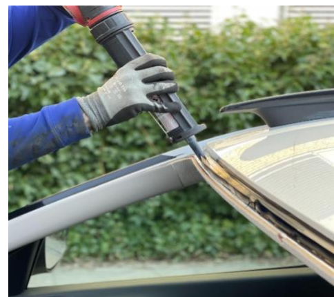
Figure 12: Applying the PUR-adhesive on a windshield frame [111]
